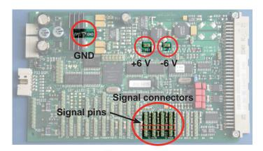
To adjust the physical zero you need to measure some voltages on the XSP board: Depending on which channel the cell is assigned to, the measuring signal (+) can be measured at pin 3 of the related connector. GND (-) is available at a separate pin (see figure).
